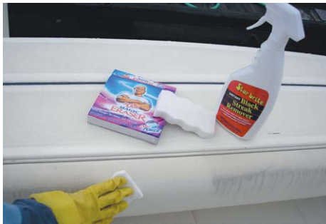
Mr. Clean Magic Eraser combined with Star-Brite's Black Streak Remover will kill water streaks.
